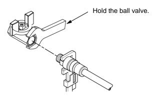
Fig. 3-19 Connection to the drain
