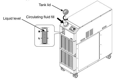
Fig. 3-21 Circulating fluid fill
