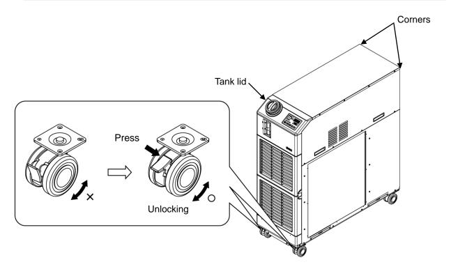
Fig. 3-2 Transportation using casters (This drawing is [HRS090-A-20].)
