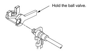
Fig. 8-5 Connection to the drain
