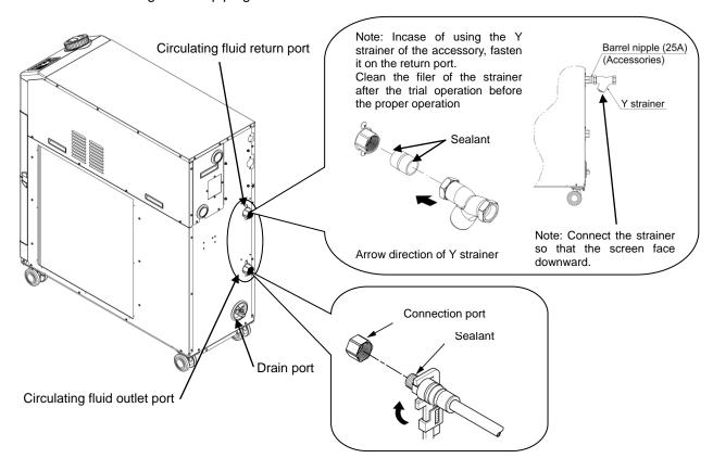
Fig. 3-18 Tightening of piping
