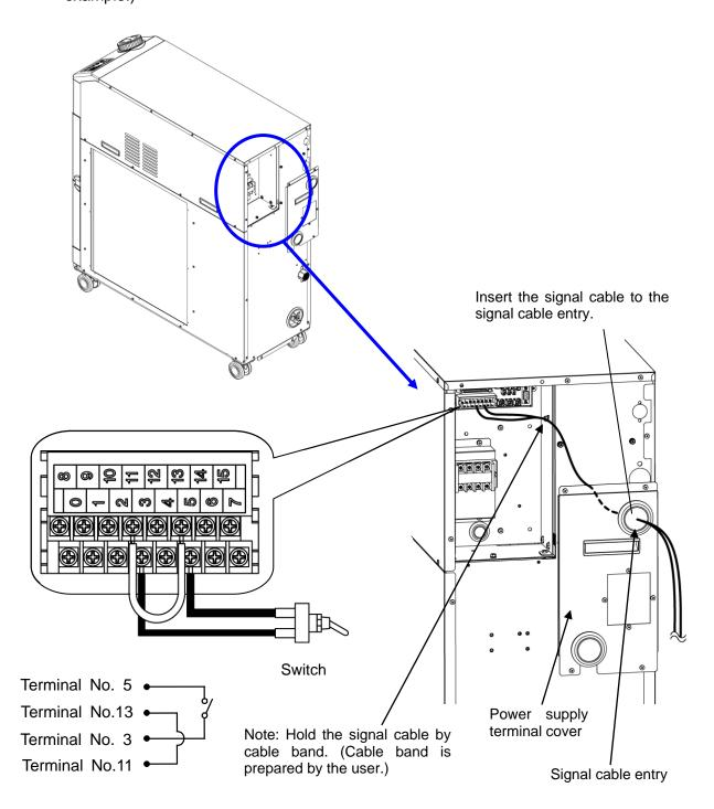
Fig. 3-13 Wiring of Run/stop signal input · Remote signal input (Example)
