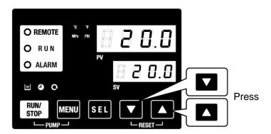
Fig. 4-2 Setting of circulating fluid temperature
