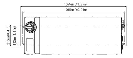
Fig. 3-6 Installation of anchor bolts
