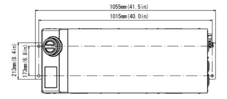
Dimensions for the positions of the anchor bolts (View a-a)
