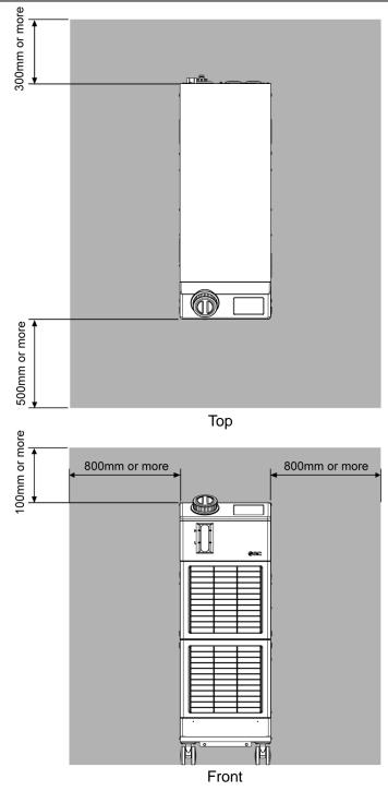
Fig. 3-3 Installation space (This drawing is [HRS090-A-20].)
