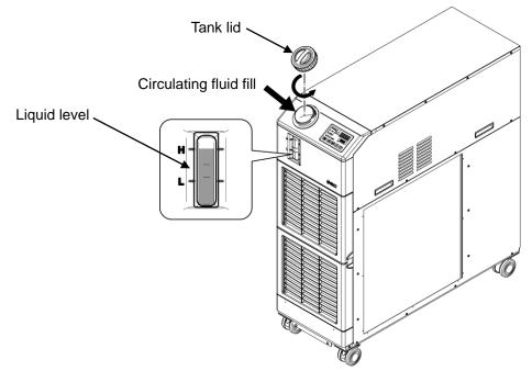
Fig. 4-6 Filling of Circulating Fluid
