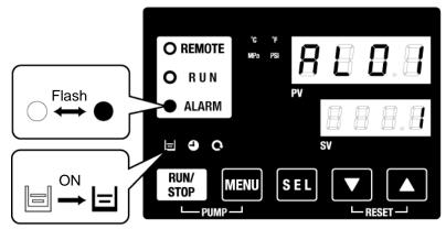
Fig. 4-4 Low tank level alarm
