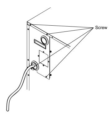
Fig. 3-12 Mounting of power supply terminal cover
