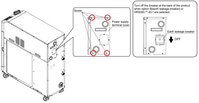
Fig. 3-8 Removal of power supply terminal cover
