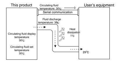
■ When only the "set circulating fluid temperature" needs to be the same as the circulating temperature supplied to the user's equipment:
