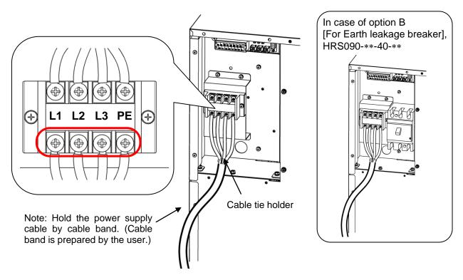
Fig. 3-11 Wiring of power supply cable
