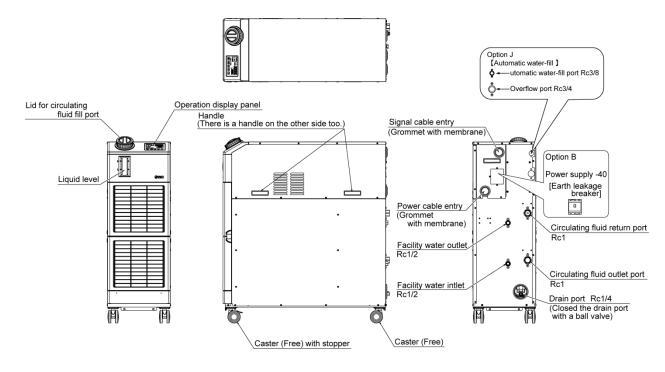
Fig. 2-3 Names of the parts (This drawing shows "HRS090-W-20".)
