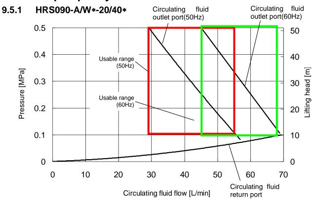
Fig. 9-7 Pump capacity (HRS090-A/W\*-20/40\*)
