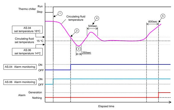
Fig 5-3 Alarm generation timing
