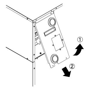
Fig. 3-9 Removal of power supply terminal cover
