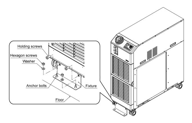
Fig. 3-7 Settlement to the floor (This drawing is [HRS090-A-20].)
