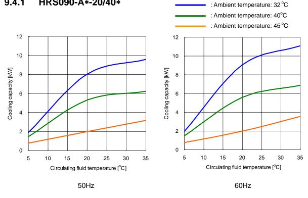
Fig. 9-5 Cooling capacity(HRS090-A\*-20/40\*)
