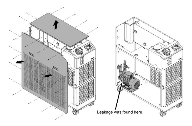
Fig. 8-3 Check for water leakage from pump
