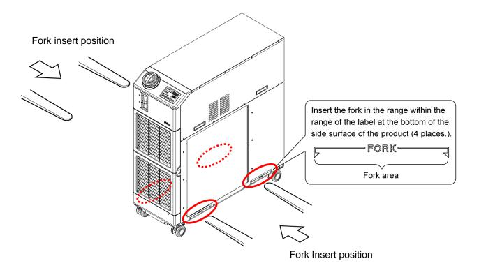
Fig 3-1 Fork inserting and hanging position (This drawing is [HRS090-A-20].)
