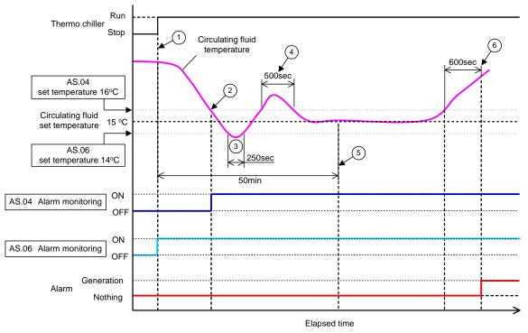
Fig 5-4 Alarm generation timing
