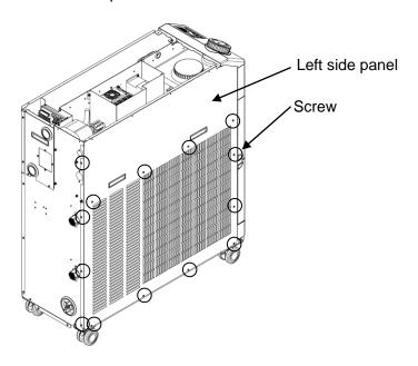
Fig. 7-5 Removal of Left side panel
