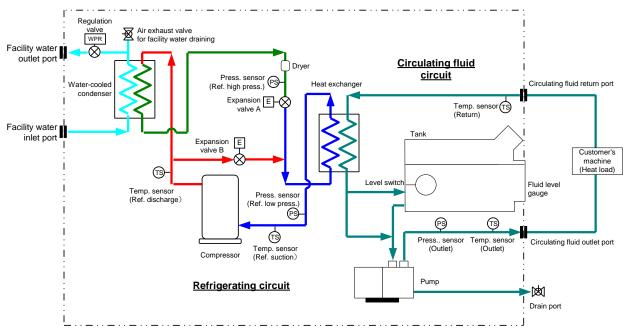
Fig. 9-4 Flow diagram(HRS090-W\*-20/40\*)
