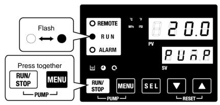
Fig. 4-3 Manual operation of the pump
