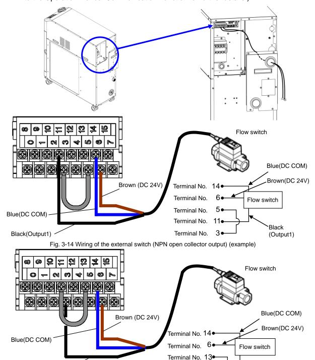
Fig. 3-15 Wiring of the external switch (PNP open collector output) (example)
