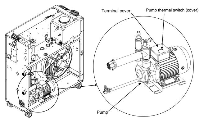
Fig. 7-6 Pump thermal switch location and statuses
