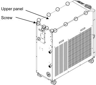
Fig. 7-4 Removal of upper panel
