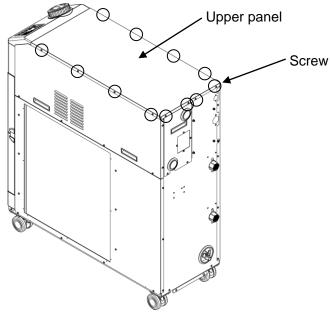
Fig. 7-1 Removal of upper panel
