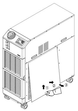
Fig. 8-1 Removal of the dust-proof filter
