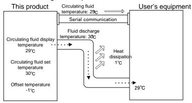
■ When both the "set circulating fluid temperature" and the "displayed circulating fluid temperature" need to be the same as the circulating temperature supplied to the user's equipment:
