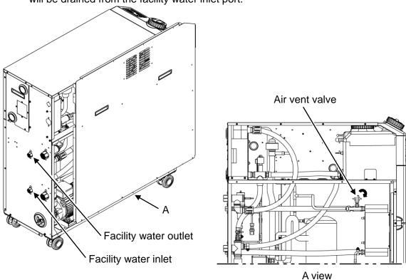
Fig. 8-6 Discharge of the facility water
