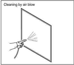
Fig. 8-2 Cleaning of the dust-proof filter
