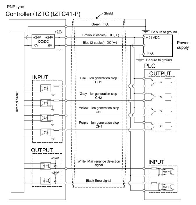
When an ionizer (IZT43) is used in DC mode, make sure to ground the F.G. cable (green) and DC(-) cable (blue) of the input power supply with a resistance of 100 ohms or less. Without grounding the DC(-) cable, this product and/or power supply may be damaged.
