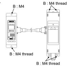
III.Adding a high voltage power supply module
