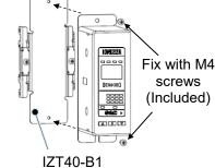
DIN rail mounting bracket for controller
