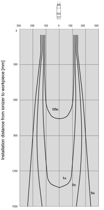
3) With Energy saving static neutralization cartridge, Supply pressure: 0.5 MPa
