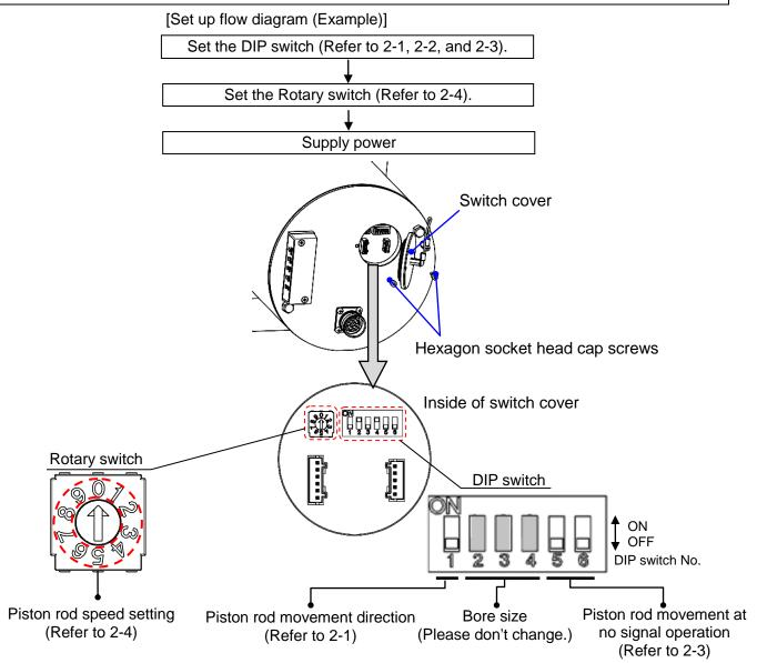
After setting, push the switch cover into the panel hole and replace the 2 hexagon socket head cap screws.(Recommended tightening torque:0.5 to 0.75 N m)
