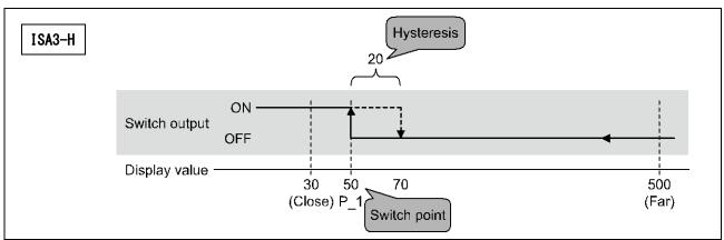
The switch output turns ON when the display value is less than switch point. (Solid line in the chart) The switch output turns OFF when the display value is greater than the switch point added to the hysteresis value. (Dashed line in the chart)
