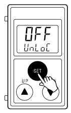
Press the UP and DOWN buttons simultaneously for <u>5 second or longer</u>. Press the SET and DOWN buttons simultaneously for <u>5 second or longer</u>.
