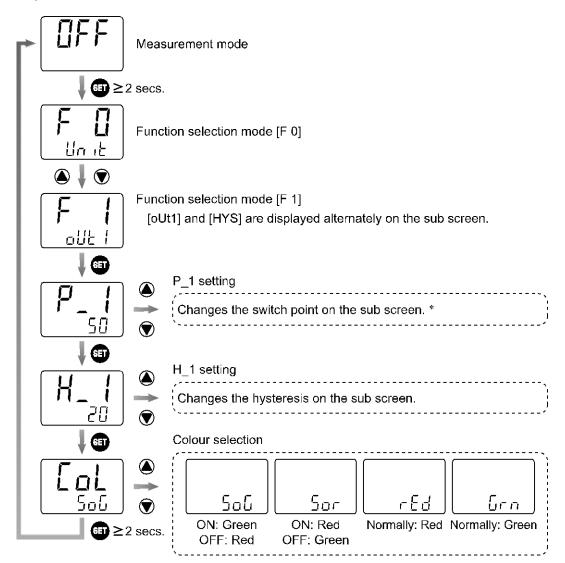
\*: The display value on the main screen can be converted to the switch point setting by pressing the (a) and buttons simultaneously for 1 second or longer and releasing them (To reduce the setting operation).
