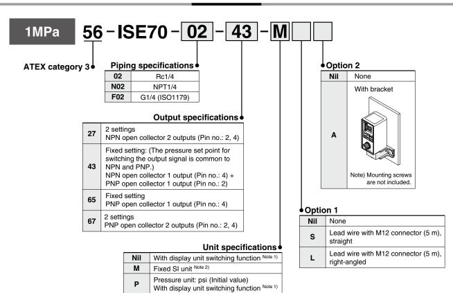
Note 1) Under the New Measurement Law, sales of switches with the unit switching function are not allowed for use in Japan. (Initial value: MPa) Note 2) Fixed unit: Mpa
