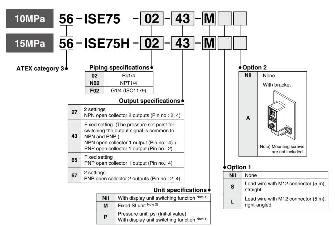
Note 1) Under the New Measurement Law, sales of switches with the unit switching function are not allowed for use in Japan. (Initial value: MPa) Note 2) Fixed unit: Mpa
