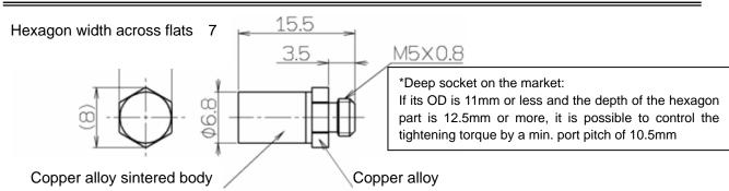
Note 1: This product cannot be used for fluids containing corrosive gas or in such atmospheres. Note 2: At the time of installation or when the product is being installed, do not apply a load to it. Note 3: For installation, after tightening by hand, rotate 1/6 to 1/4 with a tightening tool or with a tightening torque of 1 to 1.5N·m. Excessive tightening can damage the screw part.
