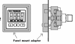
Example) Z/ISE30A can be mounted to a panel that had the Z/ISE40 or Z/ISE4 series mounted.
