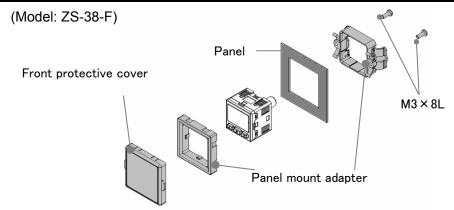
XThe panel mount adapter and the front protective cover can be rotated by 90 degrees for mounting.
