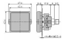
XThe panel mount adapter and the front protective cover can be rotated by 90 degrees for mounting.
