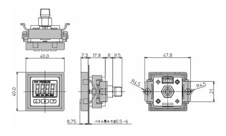
\*Panel mount adapter can be rotated by 90 degrees for mounting.
