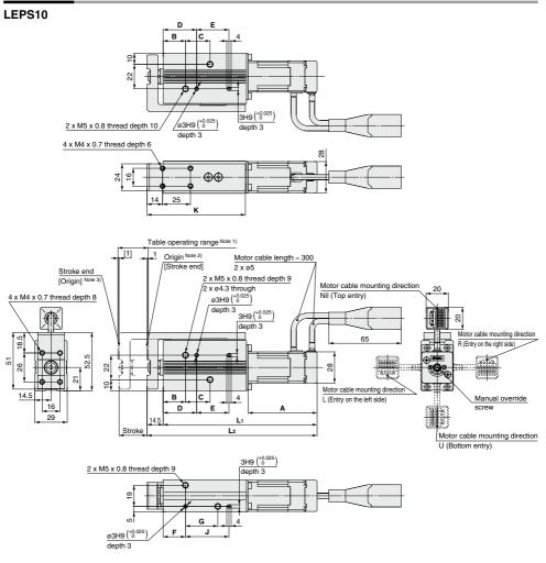
Note 1) Range within which the table can move when it returns to origin. Make sure a workpiece mounted on the table does not interfere with the workpieces and facilities around the table. Note 2) Position after return to origin. Note 3) [ ] for when the direction of return to origin has changed.
