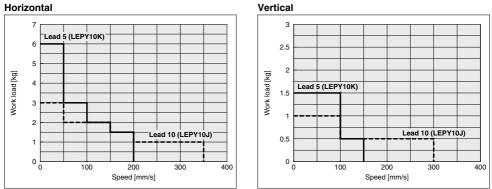
Note) The maximum value of the work load for the positioning operation. An external guide is necessary to support the load. The actual work load and transfer speed change according to the condition of the external guide.
