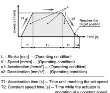
operating at a constant speed T3: Deceleration time [s] ... Time from the beginning of the constant speed operation to stop T4: Settling time [s] ... Time until positioning is completed
