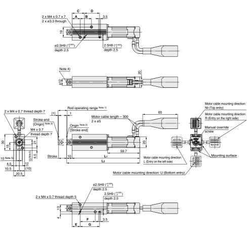
Note 1) Range within which the rod can move when it returns to origin.
