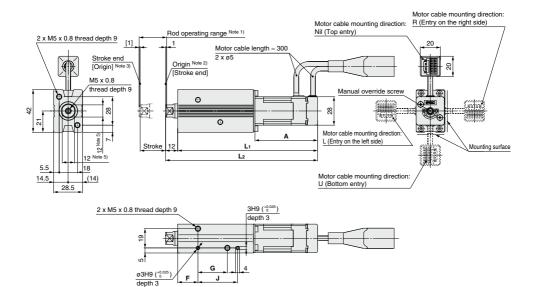
Note 1) Range within which the rod can move when it returns to origin.
