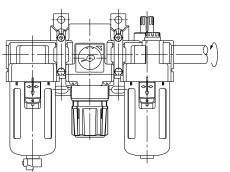
2. Avoid excessive torsional moment or bending moment other than those caused by the equipment's own weight, as this can cause damage. Support external piping separately
